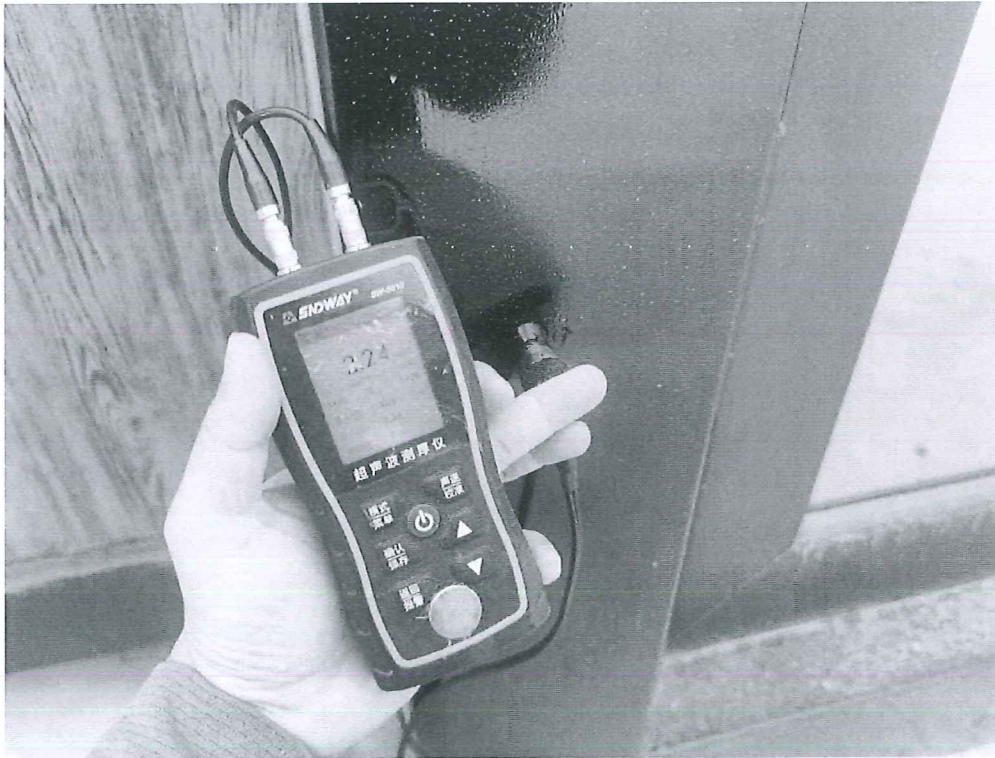
Thickness Inspection of Steel Components in the Steel Plate House
