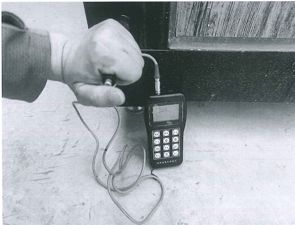
Leeb Hardness Inspection of Steel Components in the Steel Plate House
