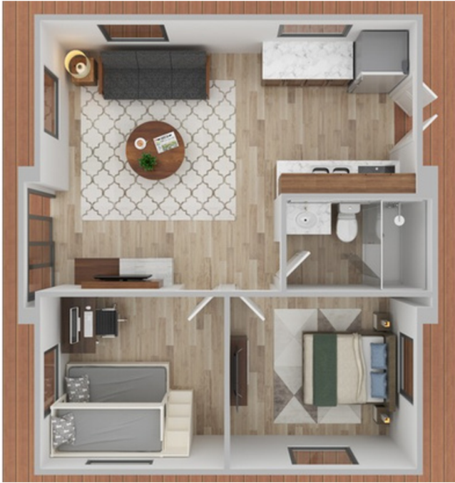
3D floor plan showcasing the layout of the 36 m 2 interior space. French door access to the verandah via the kitchen.
